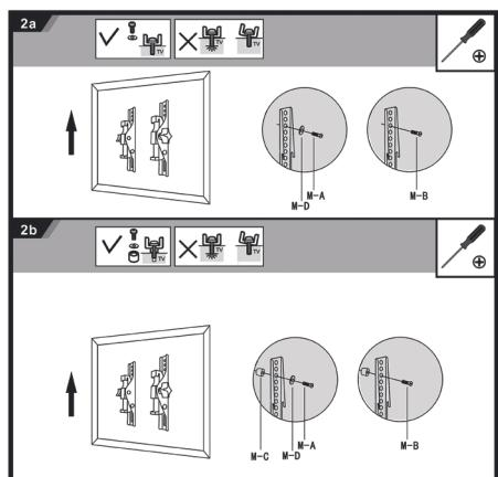
**Step 3.** Install the TV / monitor with fixed vertical profiles on the wall plate and adjust the angle of inclination. At the end of the adjustment, tighten the locking screws on the vertical profiles from the bottom.
